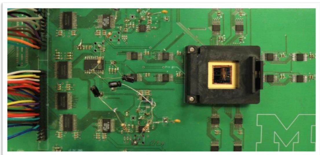
*Fig1. Memristor array situated on a circuit board.*
