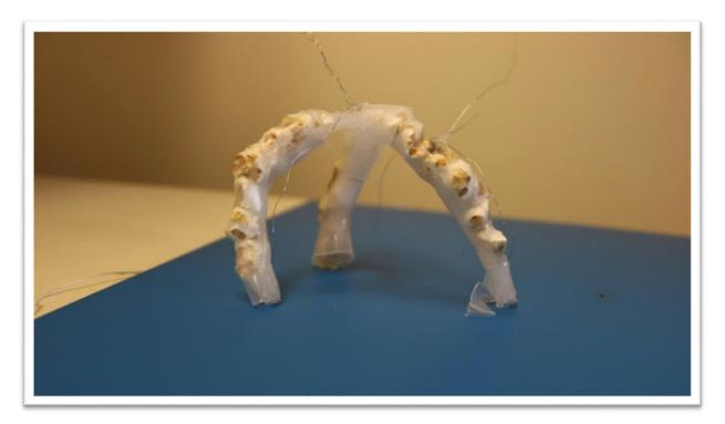
Fig 2.A soft robotic device powered by popcorn, constructed by researches in Cornell's Collective Embodied Intelligence Lab.(Credit: Image courtesy of Cornell University.)
